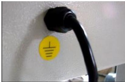
Must use socket with ground wire connected.
