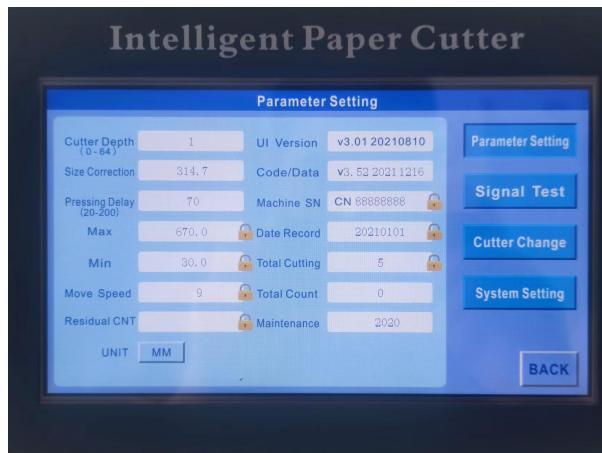
When the paper cut dimension is different from the display dimensions, you can adjust the number to fix it
